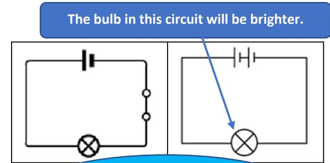
If you use a battery with a higher voltage, the bulb would also be brighter.
