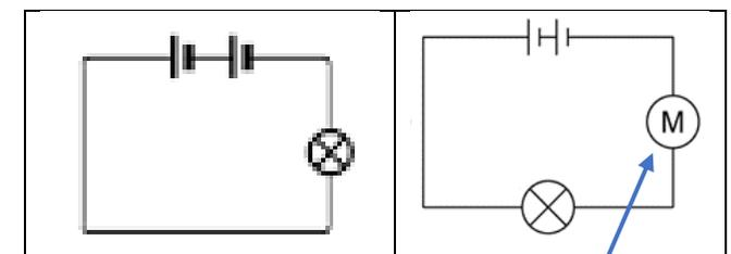
If we add a motor into a circuit with a single bulb, the bulb will be less bright.
